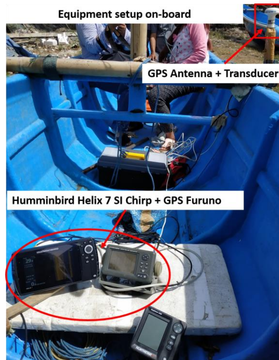
Figure 3. Equipment installation on board.
