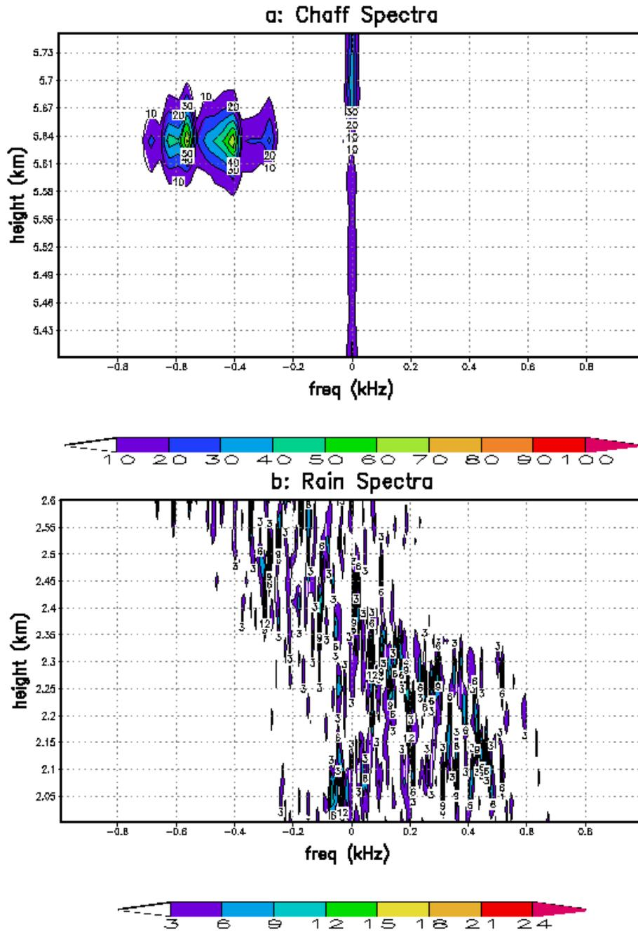
**Figure 1** Spectral comparison of chaff (a: left) and rain (b: right), notice peak values and spectral distribution on each figure
