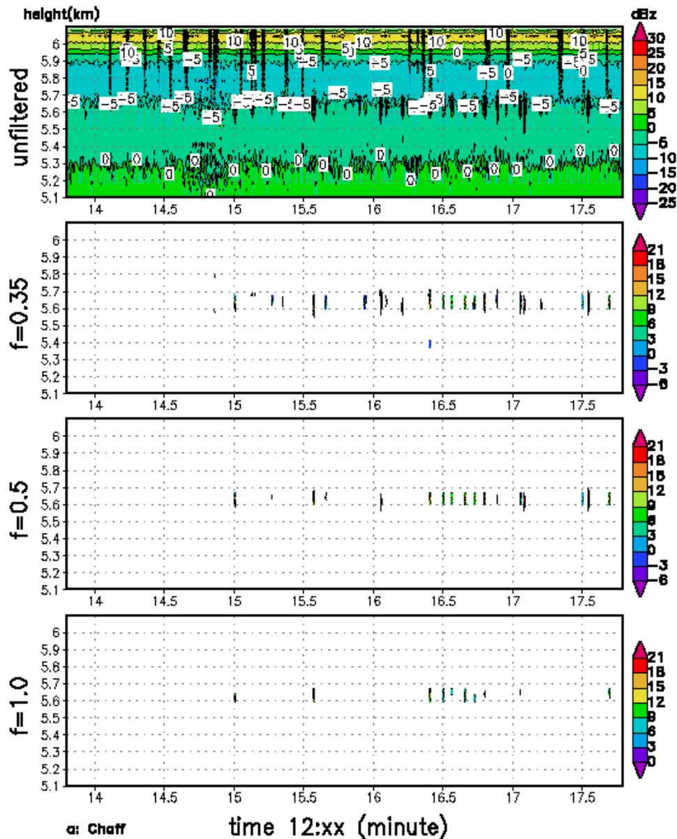
Figure 4. Filtered (a) chaff and (b) rain with different  $A_{th}$  showing filter performance. Chaff data are from November 29, 1995 and rain data from November 30, 1995. Data selected only from Zhh signatures. X-axes represents local time in minutes in indicated JST (Japan Standard Time)
