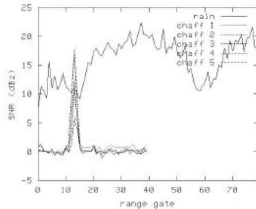
**Figure 3.** SNR of rain, chaff and simulated data, chaff only has 40 gates, while rain only shows the one above surface or up to gate 79. Rain data is taken at the extreme case (hard rain) and chaff data are taken from various experiments.
