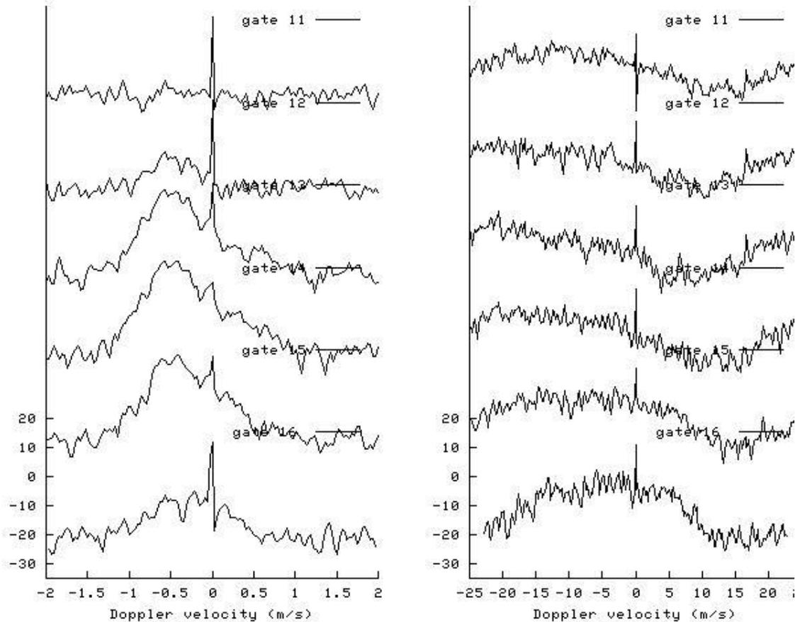
**Figure 2** Cross section of (a) chaff (left) and (b) rain (right) spectra, after 1-2-1 convolution in log scale. Most of the rain spectra show Nyquist folding as clearly located in right most part of each graph. In general, rain spectra have wider distribution
