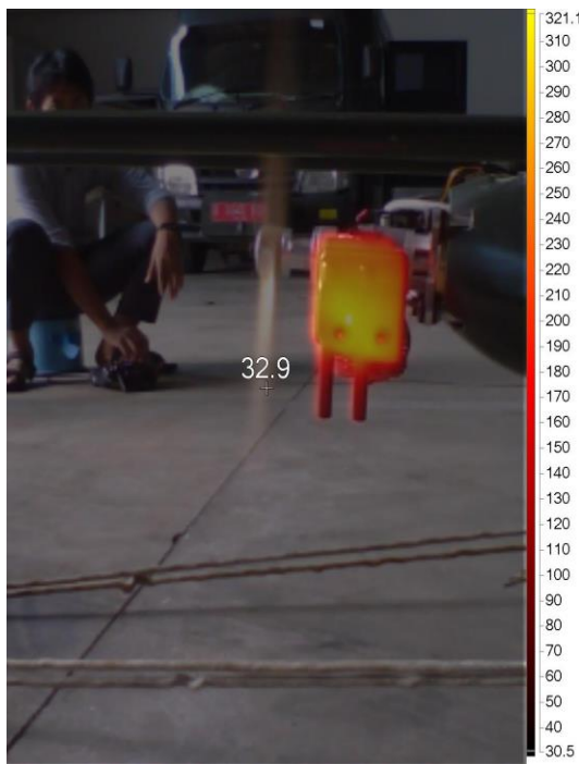
Figure 4. Temperature Contour - Exhaust Discharge (Engine and Prop)
