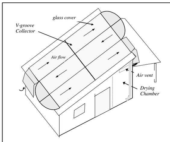
**Fig. 1. Configuration of the V-groove solar drying system**
