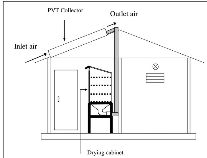
**Fig. 12. Side view of PVT solar drying system**
