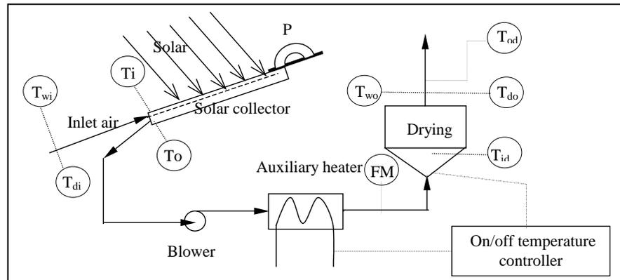
**Fig. 7. Schematic of the solar assisted drying system**
