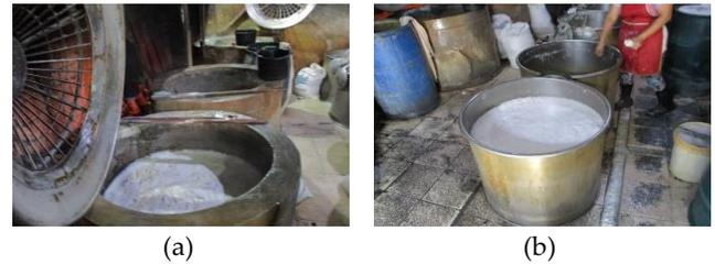
Figure 4. Tofu Industry C. Boiling tank (a), Coagulation tank (b).
