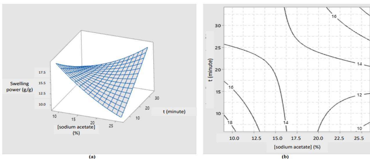
**Figure 4.** Response surface (a) and contour curve (b) for swelling power of cross-linked canna starch.
