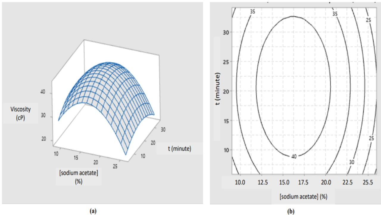
**Figure 3.** Response surface (a) and contour curve (b) for viscosity of cross-linked canna starch.
