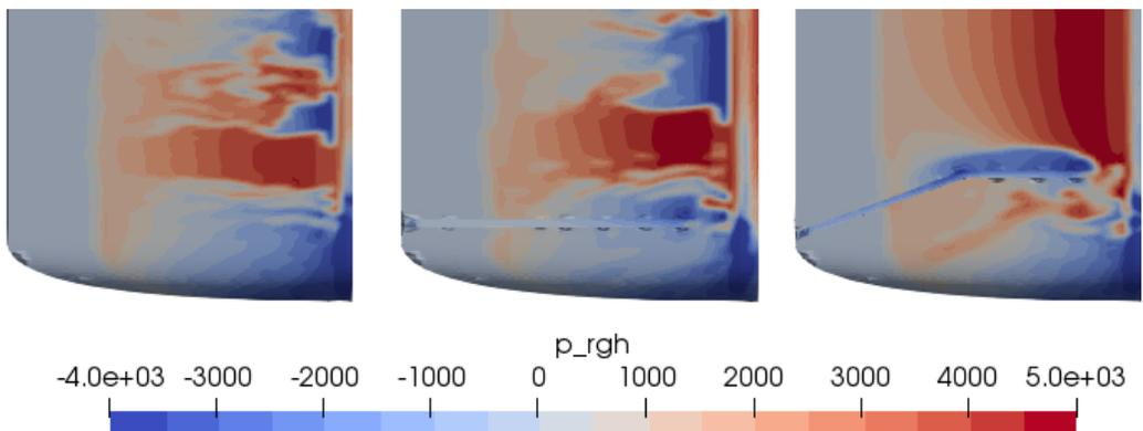
Figure 4. Dynamic pressure at barge’s stern at 50s : without skeg (left), 180° skeg (middle), 150° skeg (right)
