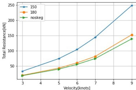
Figure 7. Barge’s total resistance
