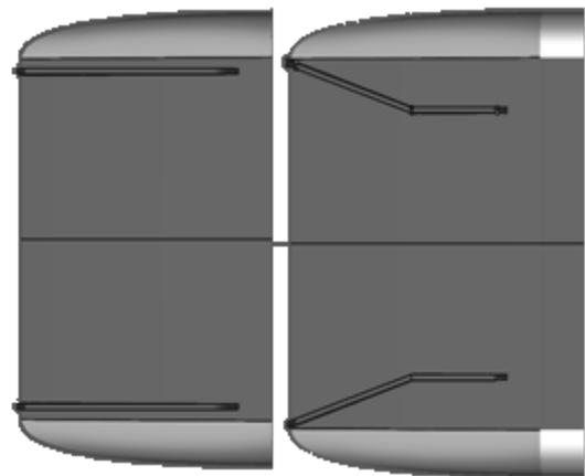
Figure 2. Skeg configuration: 180 degrees (left), 150 degrees (right)
