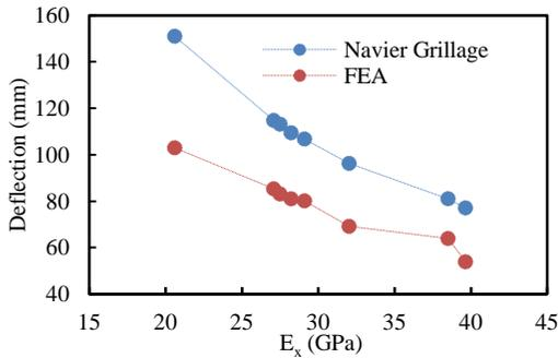
Figure 6. Deflection of composite grillages plotted against  $E_x$
