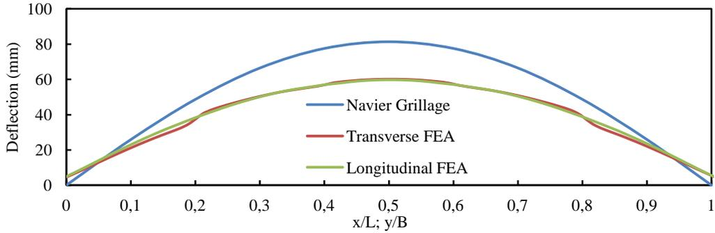
Figure 5. Comparison of deflection shape between Navier Grillage code, longitudinal stiffeners and transverse stiffener
