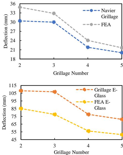
Figure 4. Deflection results of carbon and e-glass composite grillages; (Above) Carbon glass; (Below) E-glass
