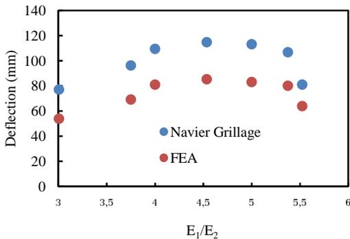
Figure 7. Deflection of e-glass composite grillages plotted against  $E_1/E_2$
