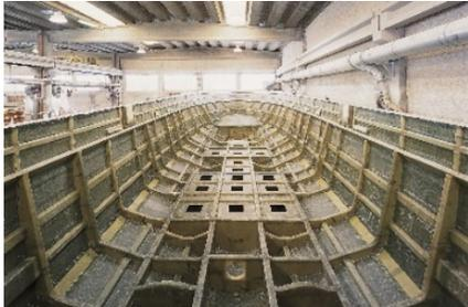
Figure 1. Grillage configuration in ship structures (Simonetta, 2019)
