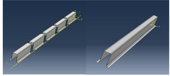
Figure 3. (Left) Transverse stiffener; (Right) Longitudinal stiffener
